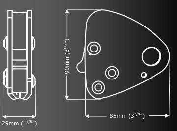
Weight 210g (7oz) Aluminium (Anodised) **Body Material** Aluminium (Hard Anodised) **Cam Material Rope Size** 10.5-11.0mm (3/8 -7/16") **Rated Capacity** 140kg (310lbs) 240kg (530lbs) Rescue (2 persons) CE EN 12841 Standards ANSI Z359.1
