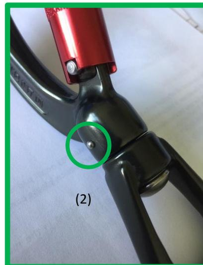
If the nut at the head of the karabiner is peened (1) or the screw through the head of the karabiner is captivated with a rivet through the body of the karabiner (2), as shown above, no further action is required at this time.
