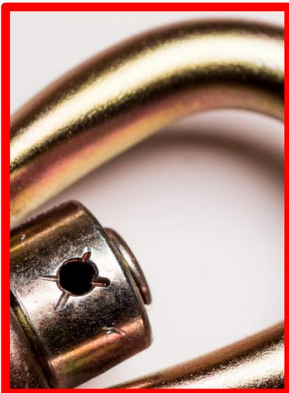
**IMPORTANT:** If you do not see the red paint or if there is no pin present or if the nut rotates or is loose the karabiner should be removed from service immediately – please return to the manufacturer in line with the corrective action at the end of this notice.
