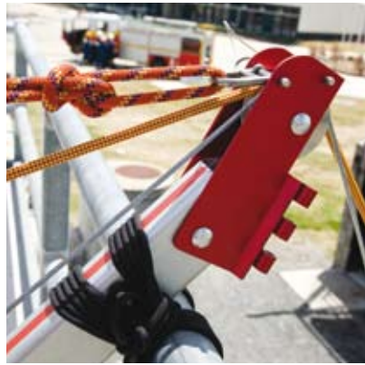
Handrail Recovery Monopole
